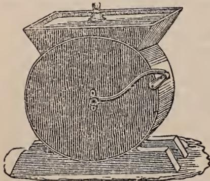
Fig. 18 is a *Cylindrical Thermometer Churn*, of any required size, with false metal bottom to hold cold or hot water for bringing the cream to the proper temperature. A thermometer, permanently set in the side, indicates the heat.
