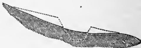
Fig. 135.—CANAL ON A HILL-SIDE.
