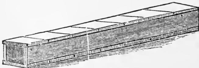
Fig. 20.—CULVERT FOR ROADS.
