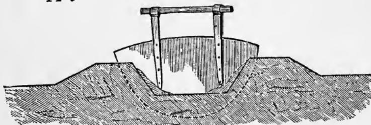
Fig. 12.—MODE OF USING HAND-GATE.
