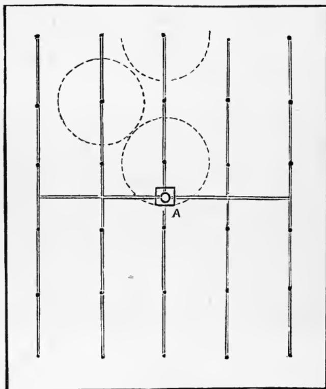
Fig. 22.—PLAN OF PIPES AND HYDRANTS.
