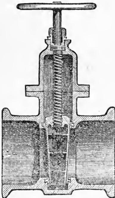
Fig. 115.—DISCHARGING PIPE VALVE.
