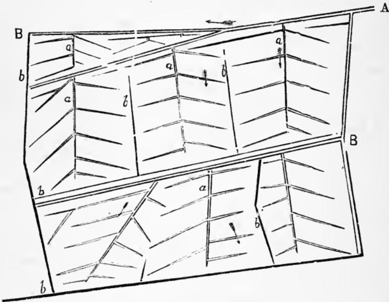
Fig. 70.—FURROWS AND DRAINS FOR IRREGULAR SLOPES.
