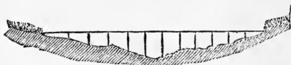
Fig. 140.—MEASURING THE CROSS-SECTION OF A STREAM.
