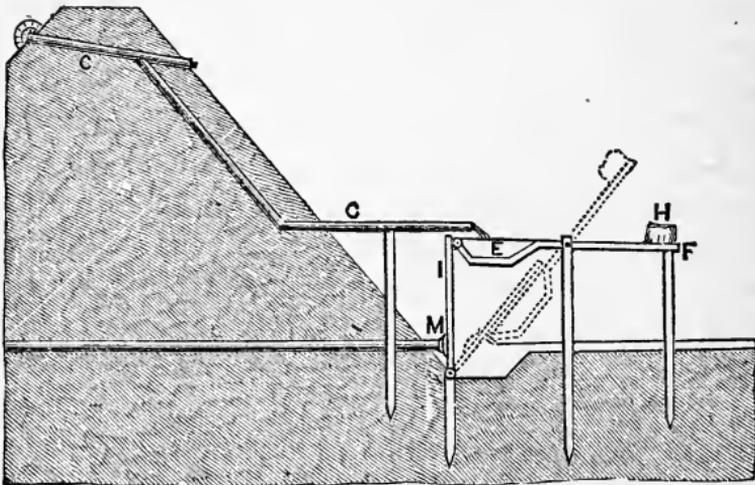
Fig. 46.—TRAP FOR DISCHARGING RESERVOIR.
