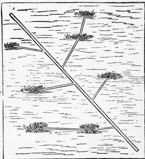
Fig. 47.—MANNER OF COLLECTING THE WATER OF SPRINGS.
