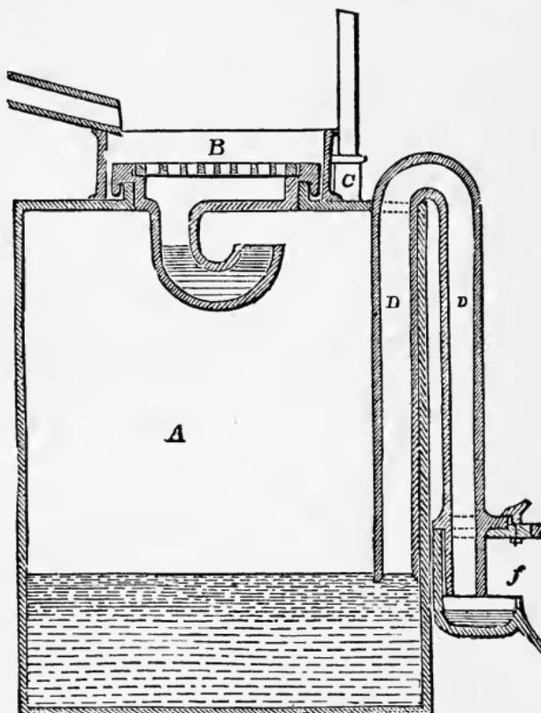
Fig. 25.—SELF-DISCHARGING SLOP-TANK.
