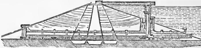
Fig. 114.—DAM WITH CULVERT AND TOWER.
