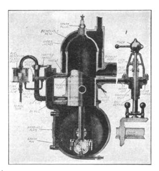
SECTIONAL VIEW OF A TWO-CYCLE ENGINE.1
