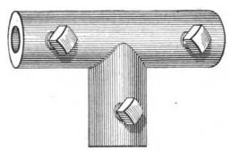
A "T" Connection for Heavy Wire Lightning Rods.<sup>1</sup>
