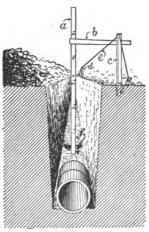
GRADING THE DITCH AND LAYING TILE.1
