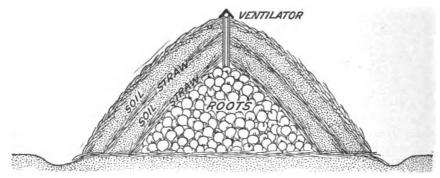
CROSS SECTION OF AN EASILY CONSTRUCTED PIT FOR ROOTS.1
