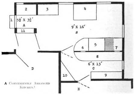
A—Cold pantry. B—Kitchen. C—Butler's pantry. D—Back hall. E—Dining room. 1—Window box to be used to keep food material in cold weather. 2—Refrigerator, with outside door for icing. 3—Kitchen cabinet. 4—Range. 5—Sink with shelves and drainage board on either side. 6—Door for passage of soiled dishes to be passed back. 7—Shelves in pantry. 8, 9 and 10—Shelves with glass doors. 11—Shelves in cold pantry.
