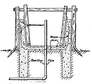
How to Construct a Concrete Water Tank.1
