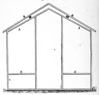
The use of the horse fork is now as much a necessity to the hay barn as the mower is to the meadow, and the frame of the modern dairy-barn should be adapted to its use, by leaving out as many as possible of the inside timbers, and by arranging those which must remain so as not to be in the way. For this purpose,
