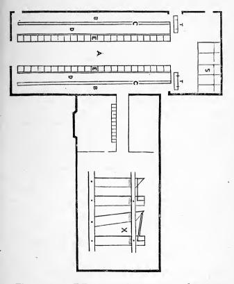
The mangers, E E, are two feet in the clear, with the bottoms raised four inches above the feet of the cow. A separate feed-box is made for each cow. It is formed by boarding up in front 16 or 18 inches, and separating their heads with a partition of two inch plank. The part over the manure shed is fitted up with stalls for transient horses and places for keeping calves in the spring, or for absorbents, as may be required.
