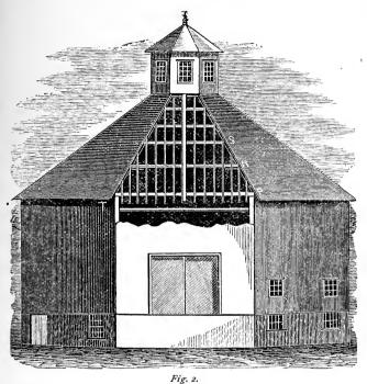
OCTAGON BARN, (NORTH ELEVATION). EXPLANATION.—P, plate; R, tie-rod and bridging between rafters; S, purlin rim: T, hip rafters.
