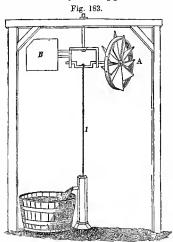
Wind-mill for pumping water on farms : A, wind-mill; B, vane; 1, pump-rod. sawing wood by the aid of a circular saw, turning grindstones, and particularly in pumping water. One of the best contrivances for pumping is represented by Fig. 183, where A is the circular wind-mill, with a number of sails set obliquely to the direction of the wind, and always kept facing it by means of the vane, B.
