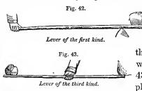
the power, as in Fig. 42, or the power may be placed between the fulcrum and the weight, as in Fig. 43, the same principle of virtual veloci-
