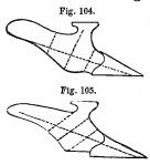
the face at right angles to the line of motion, as shown by the dotted lines in Fig. 104, the mould-board will be so far right; but if the straight edge must be placed in other positions, as in Fig. 105, it is defective in form. A mouldboard may be much modified,
