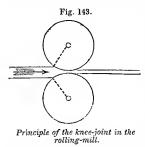
play as they revolve, are both fixed, and consequently the bar has to yield between them (Figure 143). The greatest power is exerted just as the bar receives the last pressure from the rollers. The most powerful and rapidly-working straw-outters are those which
