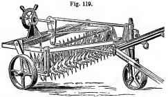
Norwegian Harrow, kept from clogging by two cylinders of teeth ploying into each other.
