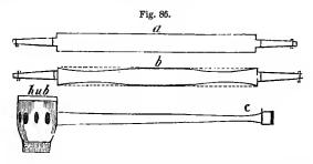
Sometimes several forces act at once on different parts. For example, the spokes of wagon-wheels require strength at the hub for stiffening the wheel; they must be strong in the middle to prevent bending, and large enough at the outer ends, where they are soonest weakened by decay. Hence there should be nearly a uniform taper, slightly larger at the middle, and with an enlargement at the outer end, as c (*Fig.* 86).
