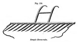
length, and draught-ropes attached. If they are too short, the teeth will be hard to guide; if too long, the rake is unloaded with difficulty. Handles serve to guide the teeth, to lift the rake from the ground in avoiding obstructions, and to empty the accumulated hay.
