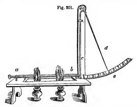
a, presses against the lever c, and this against the lever, or index, d, both of which multiply the motion, and render the expansion very obvious to the eye when the rod is heated by the lamps. If the rod should expand one fiftieth of an inch, and each lever multiplies twenty times, then the index (or second lever) will move along the scale eight inches; for 20 times 20 are 400, and 400 50ths of an inch are 8 inches.
