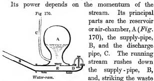
stream. Its principal parts are the reservoir or air-chamber, A (Fig. 170), the supply-pipe, B, and the discharge pipe, C. The running stream rushes down the supply - pipe, B, and, striking the waste
