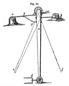
ward, and loosens the stump; while in this position, another chain is made to connect g to h, and the horse is turned about, and draws the lever backward to i, which still further increases the loosening; a few repetitions of this alternating process tears out the stump. Very strong chains are requisite for this purpose. Large stumps may require an additional horse or a yoke of oxen. Where the stumps are remote from each other, iron rods with hooks may be used to connect the chains.
