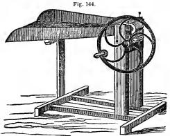
fect in this machine is its inability to cut shorter than one inch in length, which is not sufficient for cornstalks and other coarse fodder.
