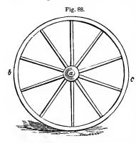
leverage of the wheel on the friction at the axis; and the smaller the axle, the greater is this leverage; for, if the axle, a (Figc ure 88), be six inches in circumference, and the wheel, b c, be ten feet in circumference, then the outer part of the wheel will move
