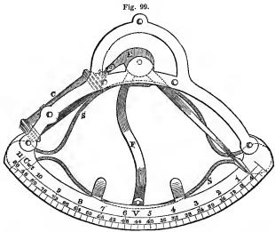
Elliptic Dynamometer, in compact form : SS, spring; F, cross-lever for moving index.
