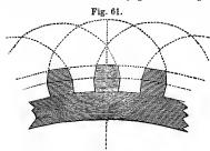
may be made as is shown in the annexed figure (Fig. 61), by striking circles whose diameter shall embrace just three teeth. The points of the teeth thus formed are removed, leav-
