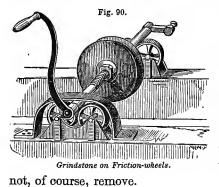
ed, for the very plain reason that, in using a grindstone, nearly all the friction is at the circumference, or between the stone and the tool, which friction-wheels could
