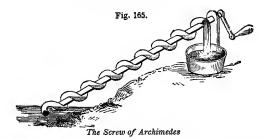
ty. Its simplicity and small liability to get out of order renders the Archimedean Screw sometimes useful where water is to be raised from an open stream to a short distance, as for irrigation, the motion being easily imparted to it by means of a small water-wheel driven by the stream.
