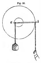
wheel be attached, so that this cord too may wind upon the larger wheel. These two wheels (fastened together so as to form one), as they are made to revolve on their axis, will now constitute, in a manner, a succession of levers, acting through an indefinite distance according to the length of the cords. The levers here successively acting are of the "first kind," and the axis of
