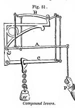
the lever A, exerting a force on the lever B five times as great as the power. B acts on the lever C with a force increased three times, and this, again, on the weight, W, with a four-fold force. Multiplying 5, 3, and 4 together, the product is 60; hence a force of one pound at P will support 60 pounds at W. By graduating (or marking into notches) the le-
