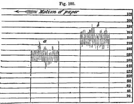
The markings of the Self-recording Dynamometer.
