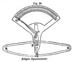
where the ends of the oval spring, Q Q, are attached to the plow and draught. The harder the force exerted by the team, the closer together will the sides of this spring be brought, causing the rod, E, to press against the index or pointer, and showing the precise degree of force on the circular scale. An improvement, by rendering the instrument more compact, is shown in Fig. 99, where S S is the spring, and directly over it is the graduated scale.
