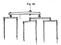
as much greater than the other as four is to three, then the weaker horse should be attached to the arm of the whipple-tree made as much longer than the other arm as four is to three.
