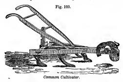
in front regulates the depth of the teeth. The width is altered by expanding or contracting the two outer beams.
