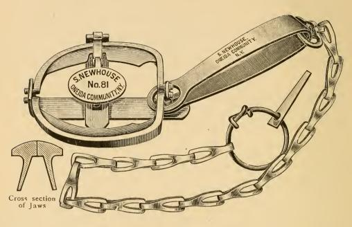
Spread of Jaws, 4 inches. Occasionally animals free themselves from traps by gnawing their legs off just below the trap jaws, where the flesh is numb from pressure. Various forms of traps have been experimented with to obviate this difficulty. The Webbed Jaws shown above have proved very successful in this respect.
