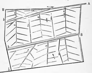
Fig. 70.—FURROWS AND DRAINS FOR IRREGULAR SLOPES.
