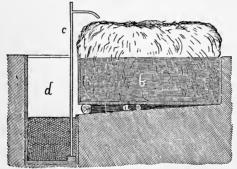
Fig. 30.—LIQUID MANURE TANK.
