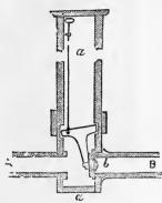
Fig. 76.—PLUG FOR CLOSING DRAIN.
