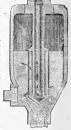
the purpose of Fig. 109.—BLUNT'S SANDlight irrigation CHAMBER.
