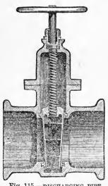
Fig. 115.—DISCHARGING PIPE VALVE.
