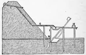
Fig. 46.—TRAP FOR DISCHARGING RESERVOIR.
