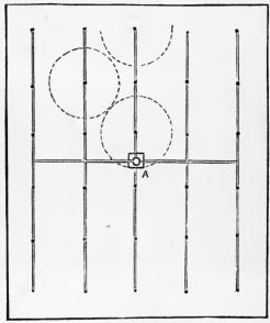
Fig. 22.—PLAN OF PIPES AND HYDRANTS.
