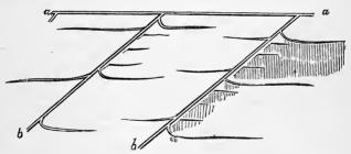
Fig. 69.—FURROWS ON A REGULAR SLOPE.
