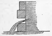
Fig. 142.—MEASURING AN INCH OF WATER.
